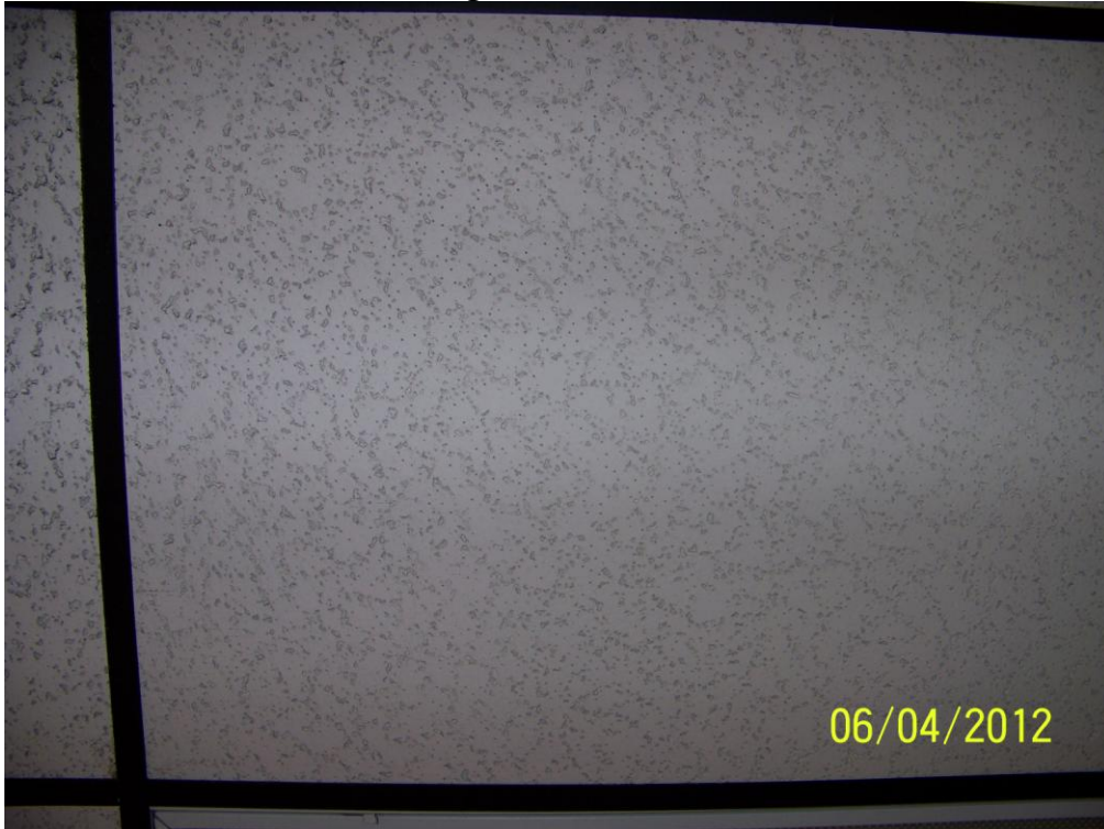
Homogeneous Material No. 11 – 2’x4’ Ceiling Tile, White, Random Pin Holes and Gouges
